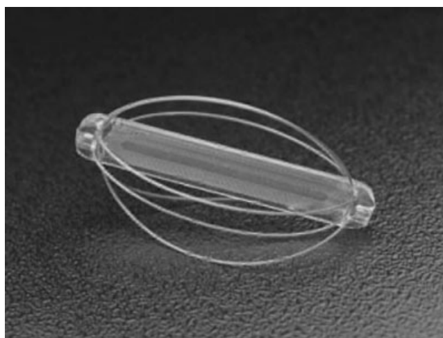
Figure 27.2 EndoSure Wireless AAA Pressure Sensor developed by CardioMems, Inc. This sensor has recently received FDA-clearance for marketing.
