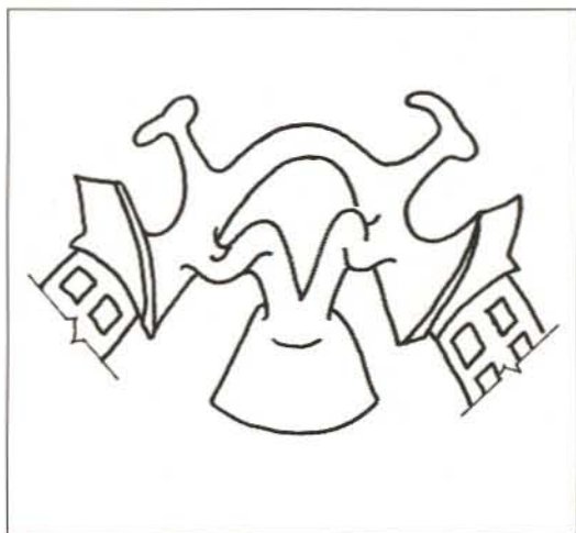
Fig 5-6 Helical sprue leads reduce turbulence.
