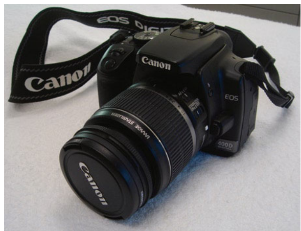
Fig. 9.1 A digital SLR camera with automatic function but also fully selectable for shutter speed, aperture, F stop, and the rest. Most of these cameras also have an interchangeable lens capability and produce an excellent image
