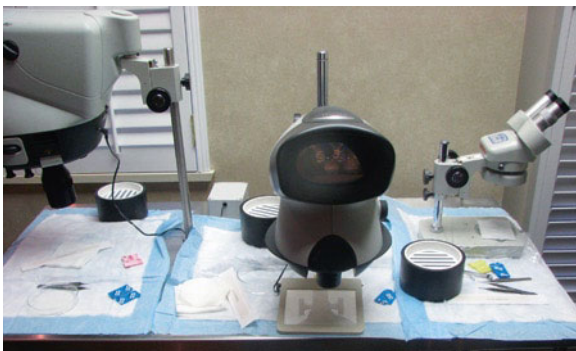
Fig. 13.23 Stereomicroscopes used in graft dissection. Meiji scope is on the right. The left and middle scopes are Mantis scopes. The middle scope is shown with an up lighter
