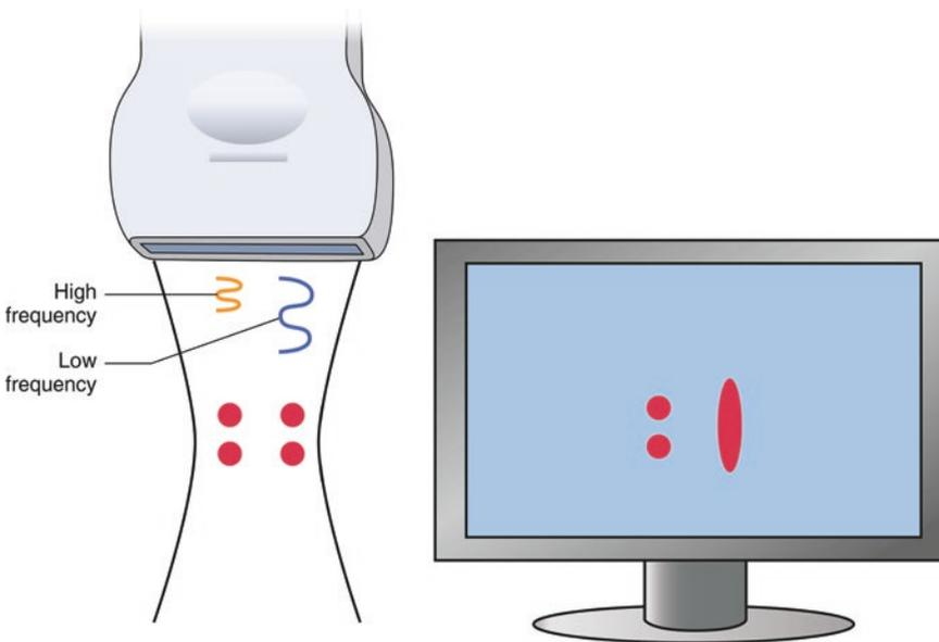
**Fig. 5.7** The effect of frequency on resolution. Higher sound frequencies require shorter pulse duration than longer frequencies. As pulse duration shortens, echoes from closely spaced objects along the beam axis become detectable. This results in better axial resolution. Lower fre-
