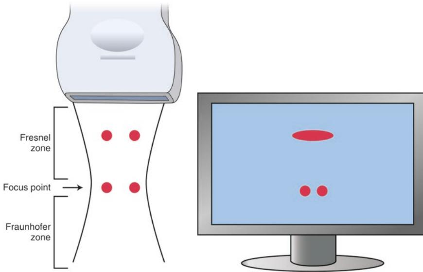
**Fig. 5.8** Narrow beam width results in better lateral resolution. Side-by-side objects within the focal zone where the beam width is narrowest are seen as separate objects on the monitor, whereas objects which had a similar dis-
