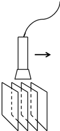
**Fig. 7.1** Multiple two-dimensional (2D) ultrasound images produced by sweeping a conventional one-dimensional (1D) ultrasound transducer over an anatomic structure of interest. The 2D images can be reformatted to display images in three dimensions (3D)
