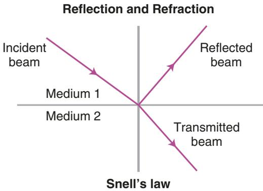
**Fig. 5.4** Snell's law. As a sound wave strikes the interface between tissues with different acoustical impedance, some sound waves are refracted and others are reflected. At a critical angle all of the waves will be reflected
