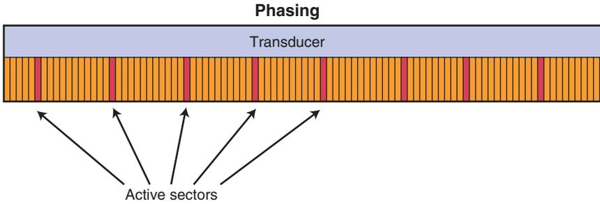
**Fig. 5.6** Graphical depiction of an array transducer. A transducer is made up of numerous small, independently controlled crystals. Firing of each crystal can be con-
