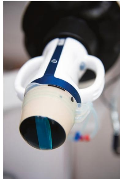
**Fig. 36.6** The VTU contains both the ultrasound imaging transducer (7.5 MHz) and the HIFU transducer (3 MHz) for delivering the energy to the target. A cooling circuit specific for the device turns down temperature among consecutive pulses
