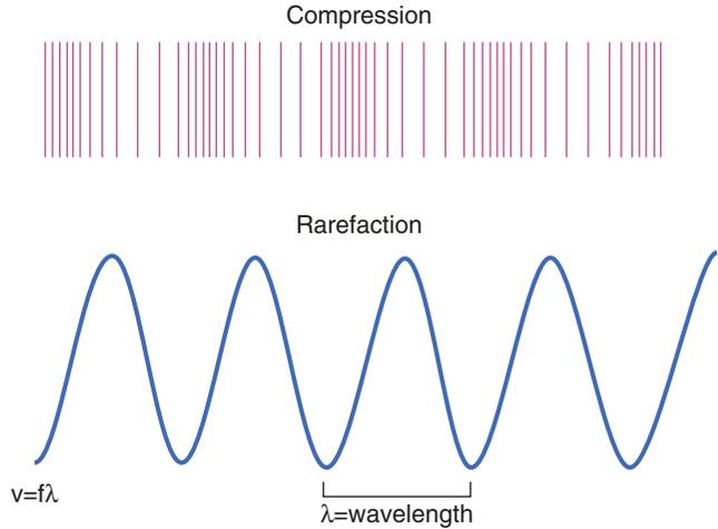
**Fig. 5.2** Velocity ( $V$ , or often noted as  $c$ )=frequency (in cycles/second)  $\times$  wavelength ( $\lambda$ , distance/cycle). For a given velocity (determined by the medium), a higher frequency is accompanied by a shorter wavelength. The *top* sine wave represents sound with a longer wavelength and lower frequency as compared with the *bottom* sine wave which depicts a higher frequency wave with shorter wavelength
