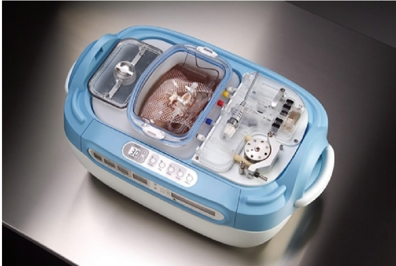
FIGURE 9.8 A portable LifePort™ hypothermic kidney perfusion apparatus. The LifePort™ Kidney Transporter, a portable hypothermic perfusion device (Organ Recovery Systems, Des Plaines IL), opened to show the kidney placed in the sterile disposable cassette (center). The system comprises online recording for renal temperature, pressure, and flow. The perfusion solution is KPS-1, Belzer's Kidney Perfusion Solution with HES (see Table 9.7). Photo provided by Organ Recovery Systems.
