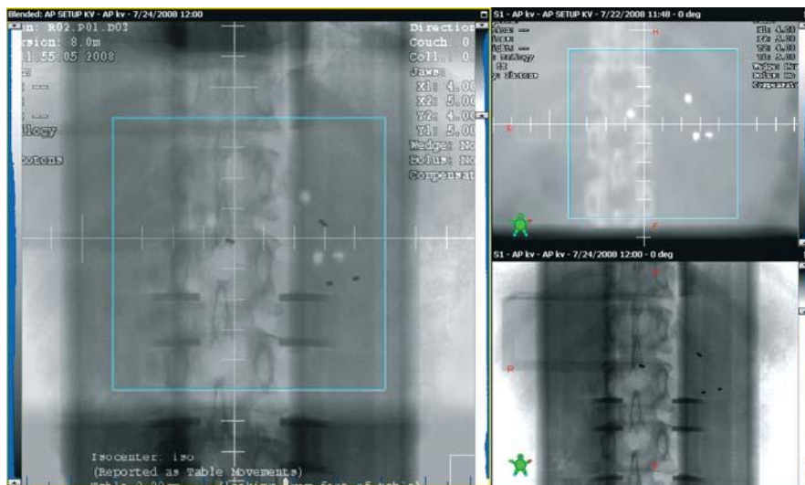
FIGURE 2.13 kV–kV image matching using high-atomic-number implanted fiducials. Two orthogonal kV images taken prior to treatment are superimposed on the corresponding DRRs obtained from the CT images used for treatment planning. The fiducials are seen on both sets of images (white dots on the DRR images, black dots on the kV images). The software calculates patient shifts in the x , y , and z directions to achieve the desired match. (Courtesy of Radiation Oncology Department, Lahey Clinic.)
