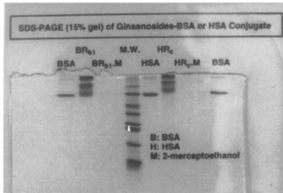
Fig. 4. Gel electrophoretogram(PAGE 15%) of ginsenoside-protein conjugates.
