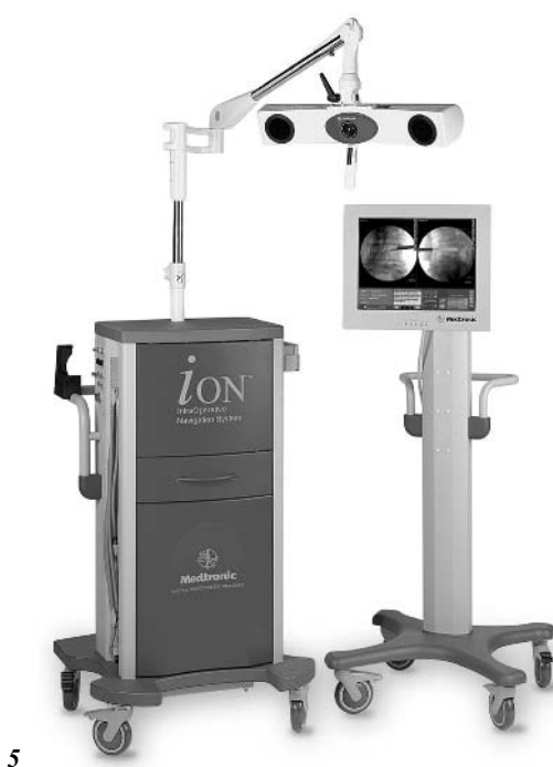
Fig. 5. The Fluoronav system (Medtronic Sofamor Danek) includes a workstation with a high-powered computer and a high-resolution monitor, an optical camera, and an attachment with LEDs and fiducial display for the C-arm.
