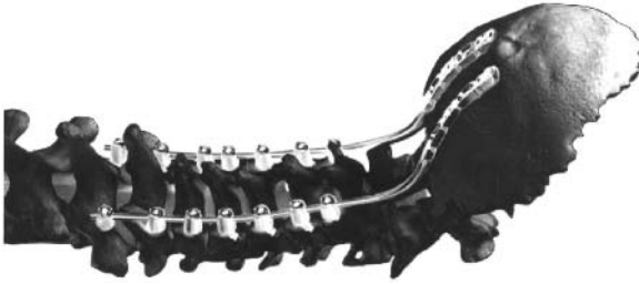
Fig. 6. Photograph of occipitocervicothoracic fixation in a saw bone model utilizing the VERTEX system.
