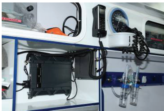
Picture 5. A view of the communication terminals inside the ICU ambulance.
