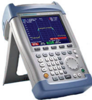
Fig. 4. Spectrum analyzer Rohde & Schwarz FSH6
