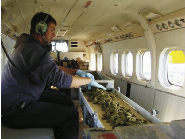
FIGURE 4 Photo of MNR staff in the back of a Twin Otter aircraft operating OES software controlled baiting machine to aerially distribute ONRAB ® baits in Ontario during September 2009.
