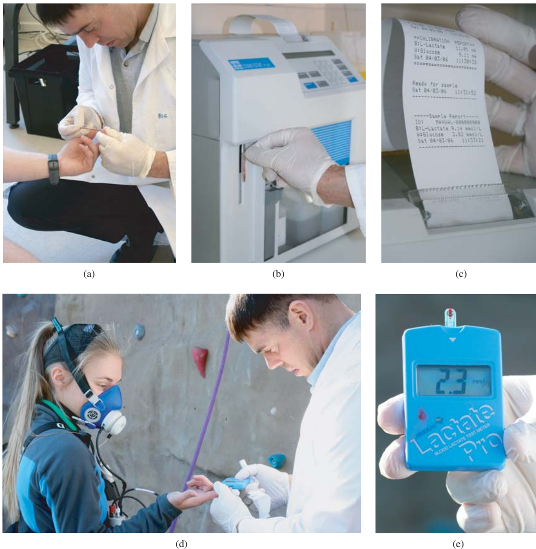
Figure 7.5 Laboratory and field measures of capillary lactate concentration: laboratory analysis depicting (a) blood sampling, (b) introduction of the sample for analysis and (c) printout of result; field analysis showing (d) blood sample being taken from a climber and (e) readout obtained in the field
