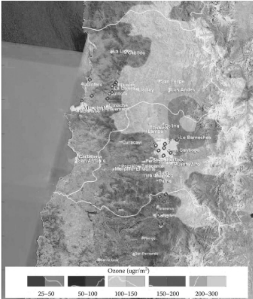
FIGURE 3.4 Mean simulated daily maximum ozone concentrations in Central Chile, January 1–15, 2008, using WRF-Chem at 3 km resolution. (From Park O.H. and Seok M.G., Atmospheric Environment , 41, 2007. 6095–6101. With permission.)
