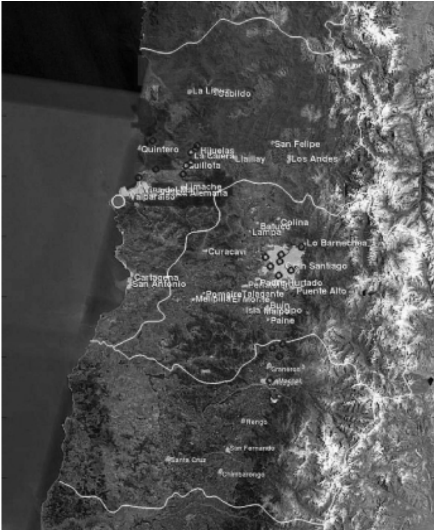
FIGURE 3.5 Influence of a large power plant on ozone formation, calculated as the difference between modeled ozone with and without emissions from the source. Light shading denotes an increase in ozone concentration greater than 1 \mu\text{g}/\text{m}^3 ; dark shading denotes a decrease in ozone concentrations. The dot denotes the location of the point source. WRF-Chem at 3 km resolution was used.
