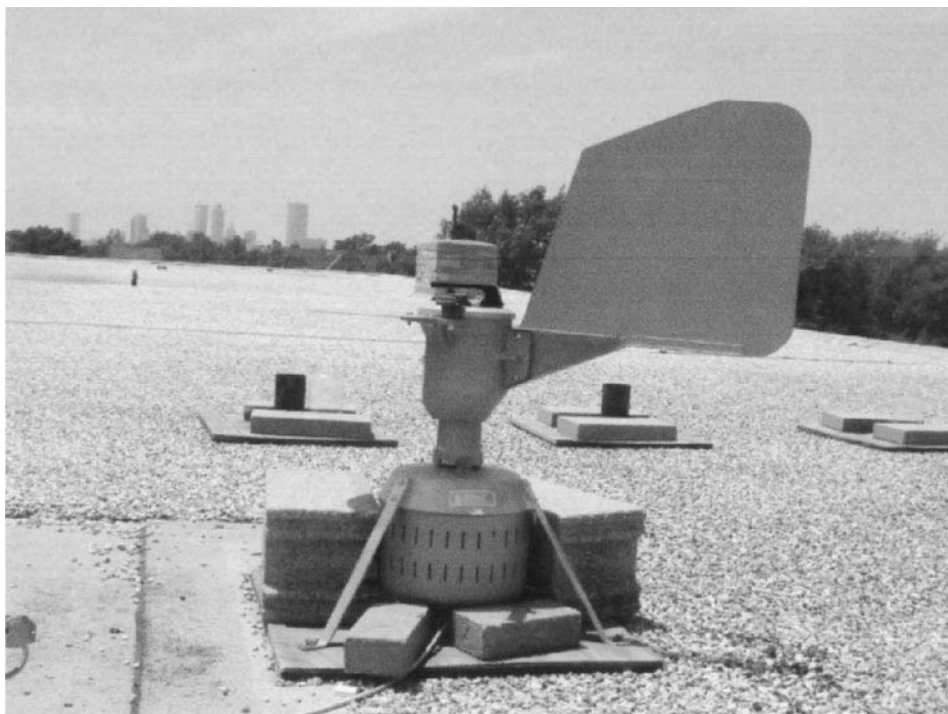
Figure 1 Recording Burkard spore trap (suction-type impactor) installed on a rooftop. This sampler can be configured to record for 7 days or for 24 hours.
