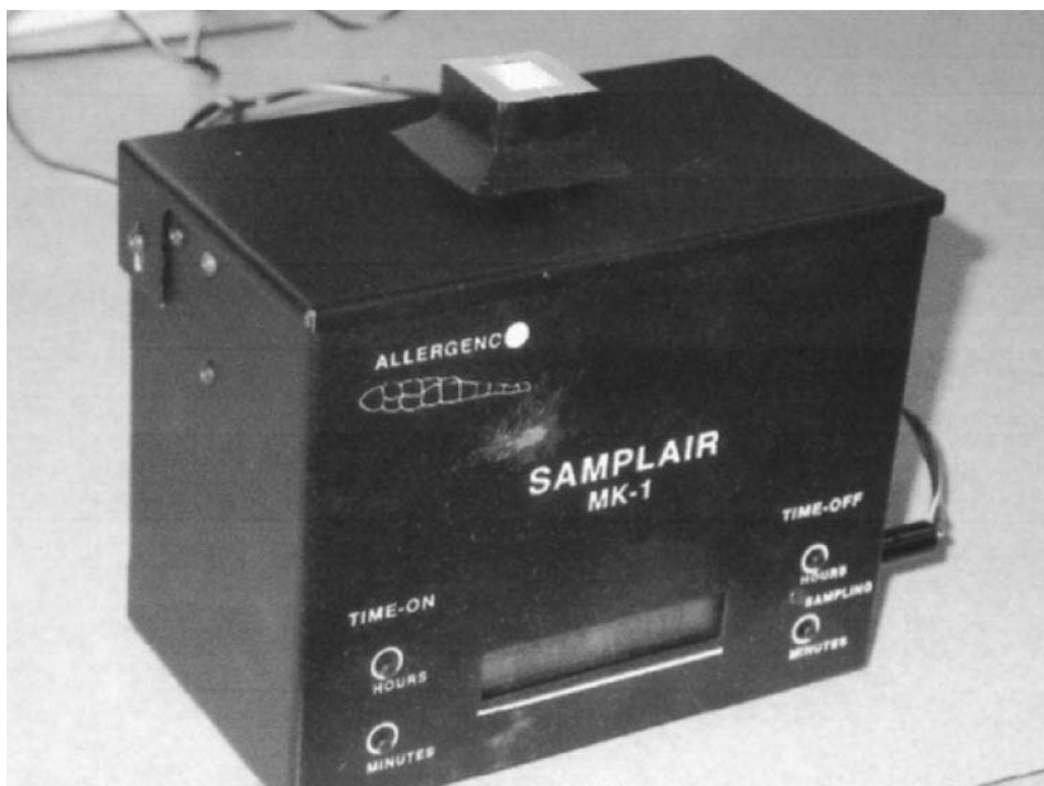
Figure 2 Allergenco suction-type spore trap. This sampler collects multiple, discrete samples at predetermined intervals and can be used to monitor outdoor trends or for indoor investigations.
