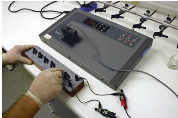
Fig. 13.2 Calibration of the Wheatstone bridge apparatus
