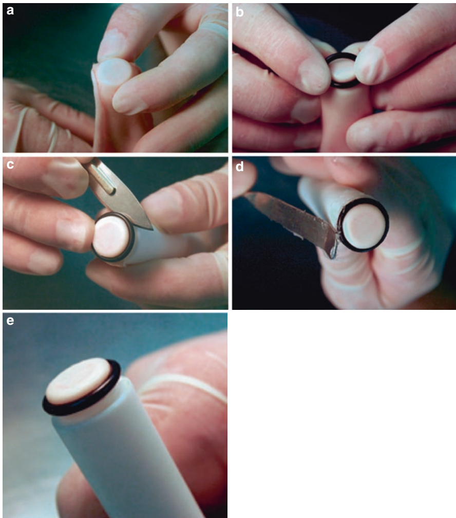
Fig. 13.4 (a–e) Skin disc preparation. (a) The prepared skin is placed over one end of a PTFE tube, epidermal surface in contact with the tube. (b) A rubber 'O'-ring is press fitted over the end of the PTFE tube. (c) Excess skin is trimmed away. (d) 'O'-ring is sealed using petroleum jelly. (e) Skin disc in situ
