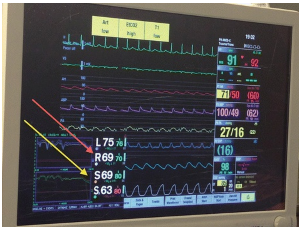
Fig. 15.4 Typical standards of monitoring in patients undergoing lung transplantation [EKG, invasive BP (Femoral-Purple, Radial-Red), pulmonary arterial pressure (yellow), central venous pressure (blue), pulse oximetry, capnography, temperature, and cerebral (red arrow)/leg (yellow arrow) near infrared spectroscopic oximetry (arrows)]
