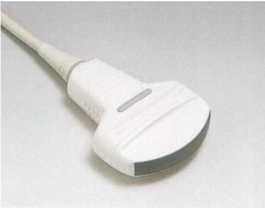
Fig. 20.1 Traditional convex probe with 3.5 MHz frequency
