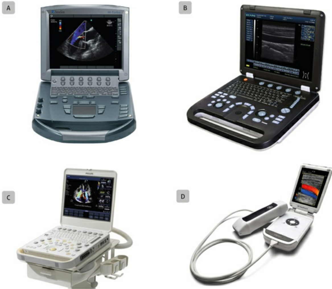
Fig. 15.1 . Portable ultrasound systems. Different ultrasound machines are shown including the (A) Sonosite M Turbo; (B) General Electric Vivid I; (C) Philips CX 50; (D) General Electric handheld Vscan 3rd generation.
