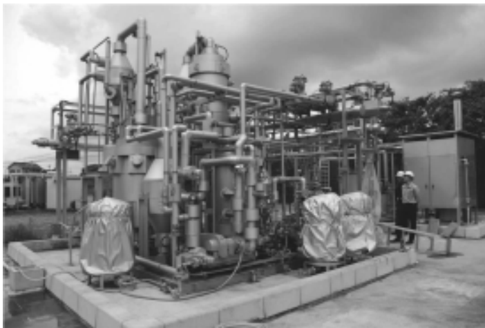
FIGURE 16.6 Demonstration plant based on the superheated methanol vapor bubble method (design productivity: 400 L/d).
