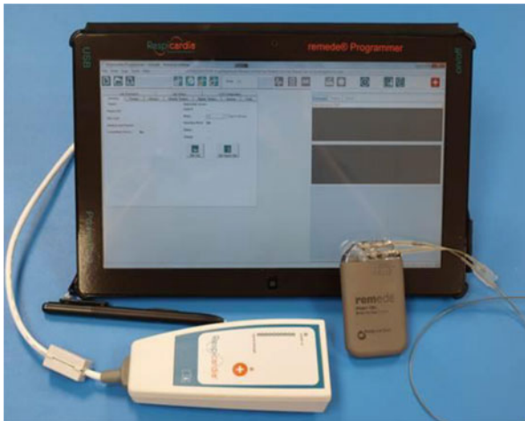
Fig. 13.4 The remedē® System consists of an implantable pulse generator, an implantable stimulation leads, and an external system programmer
