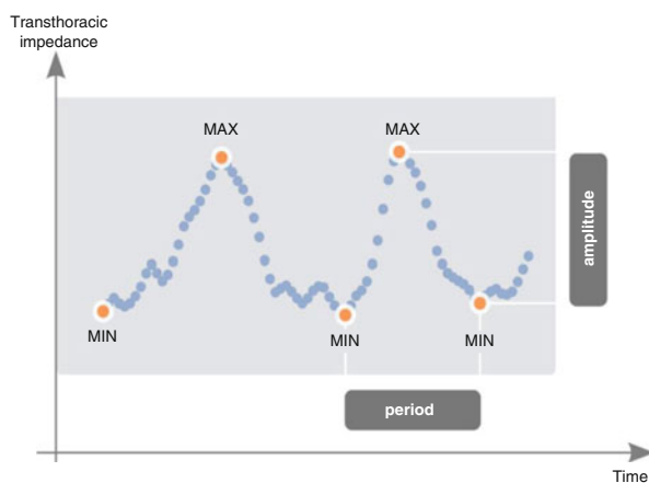
Fig. 11.5 Measure of MV in dynamic impedance: for each cycle (inspiration-expiration), the sensor measures a MIN (+) and a MAX (+) value, extracting an AMPLITUDE, and a PERIOD (Courtesy of LivaNova)
