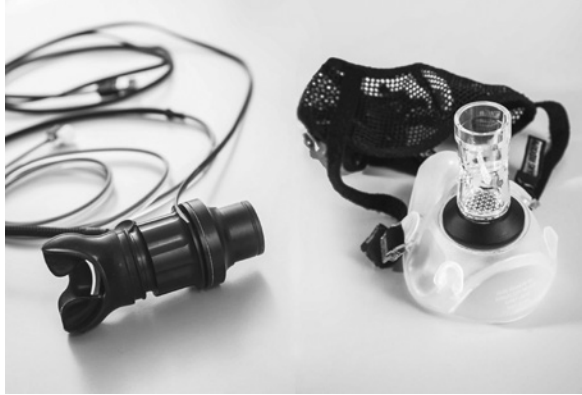
Figure 7.3 A turbine with a mouthpiece and a pneumotachograph with a face mask.
