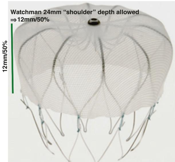
**Fig. 6.9** Watchman device: the fabric covers 50% of the height of the device; a shoulder of around 12 mm can be accepted for a 24 mm device
