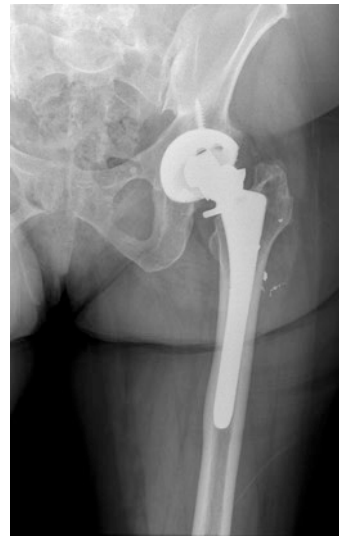
Fig. 20.8 AP and lateral radiographs of the left hip demonstrating a ceramic ball head fracture. Notice the loss of sphericity and fragmentation of the femoral head. These particles are extremely sharp and abrasive and must be removed to prevent subsequent third-body wear
