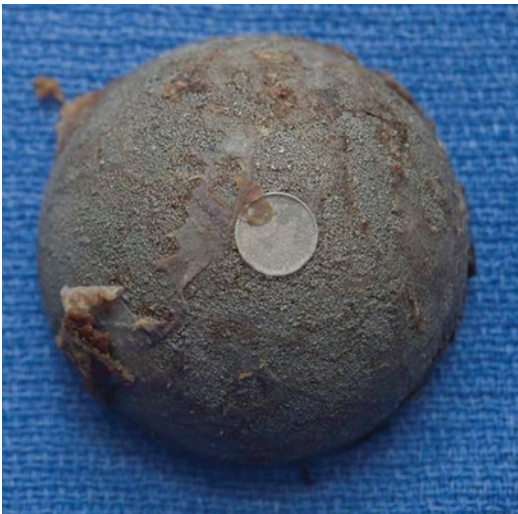
Fig. 15.10 Retrieval of fibrous ingrown ASR cup at the time of revision
