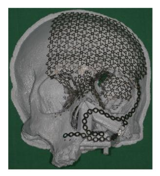
**Fig. 2.33** Rapid prototyping of the defect reconstruction including dental implants and CAD titanium implants
