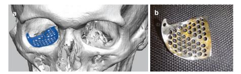
**Fig. 16.2** (a) Virtual 3D image of orbital floor reconstruction mesh plate to repair orbital wall fracture. A lateral ledge was designed to guide the plate into right anatomic position during the surgery. (b) The solid titanium plate manufactured using direct metal laser sintering technique; note the lateral guiding ledge
