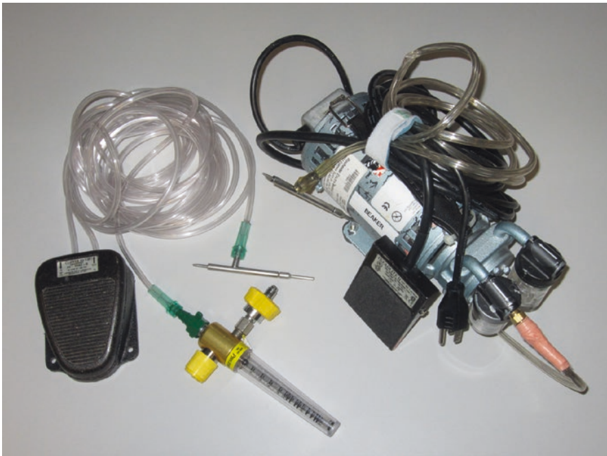
Fig. 2 Example of devices that are used to dry glue. ( Left ) An air regulator, tubing, pedal, and stylist connect to medical air in the room. ( Right ) An electric air pump with tubing, pedal, and stylist eliminate the need for medical air to be present in the room
