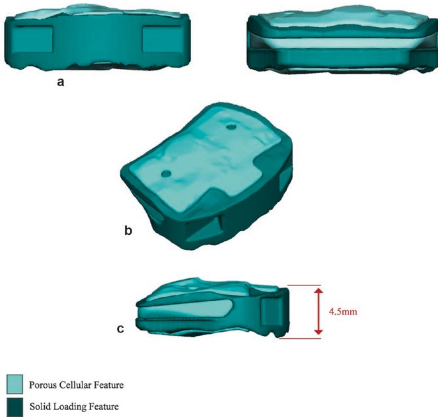
**Fig. 11.6** Final design of the individual implant (anteroposterior view **(a)**, oblique view **(b)**) demonstrates the individualised surface of the cage exactly mimicking the anatomy of the patient's endplates. **(c)** A lateral view shows the 4.5-mm measurement of the ventral disc height
