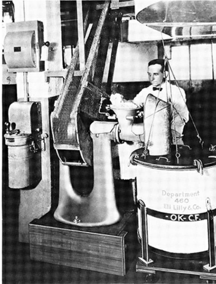
Grinding pancreas to make insulin at Eli Lilly's Indianapolis plant, 1923. Eli Lilly and Company Ltd.
