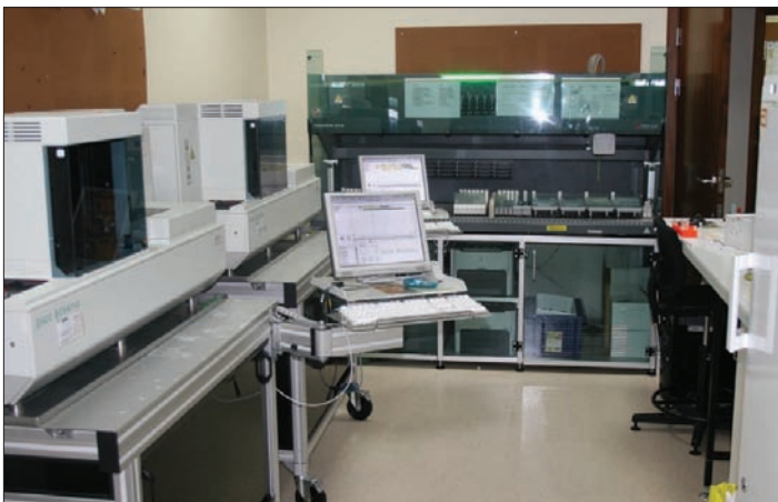
2.19 Serodiagnosis (looking for microbial antigens or antibodies) by immunoassay is carried out by automated analysers in batches with a rapid turnover time for results.
