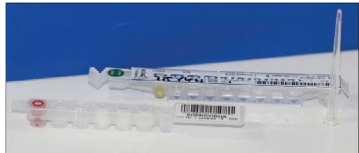
2.20 Immunoassay strip for adenovirus and HIV with wells for the various reaction steps that are carried out by the analysers.
