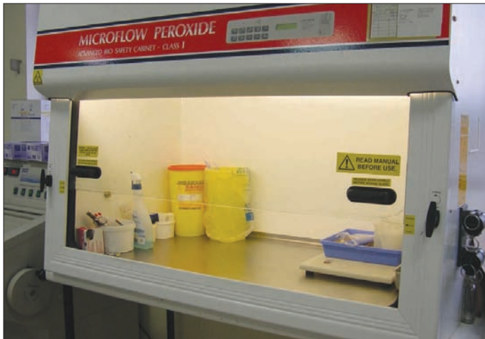
2.13 Biological safety cabinet (BSL1 or 2) in a routine diagnostic microbiology laboratory for containment of aerosols produced while processing a specimen. A higher biosafety level is applied for stringent conditions depending on the degree of biohazard of the suspected microorganism.
