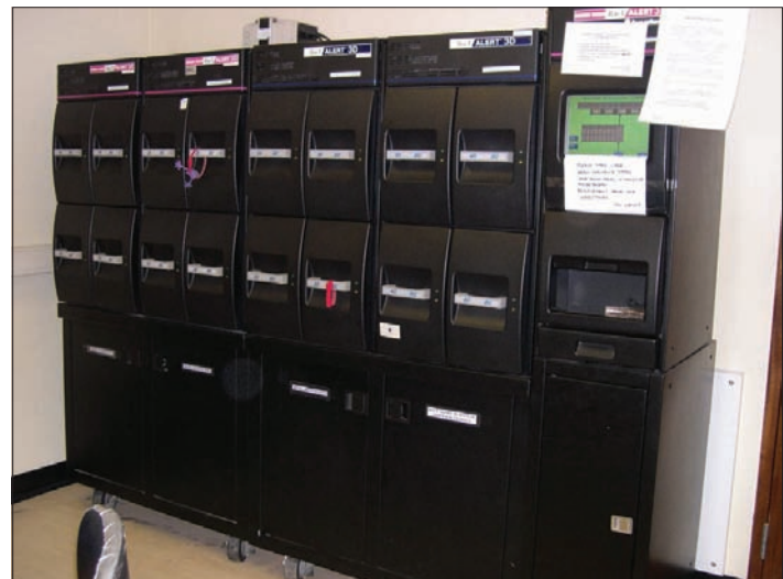
2.12 Blood culture system. This consists of cabinets with receiving wells for blood culture bottles. As microorganisms grow, liberated carbon dioxide is detected by a colour changing sensor that sets off an alarm alert. Gram stain and culture of the blood is performed on the positive culture bottles.
