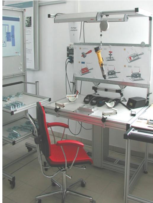
**Ergonomics and Demographics, Fig. 4** Model workplace for an assembly task (Source: IAG)
