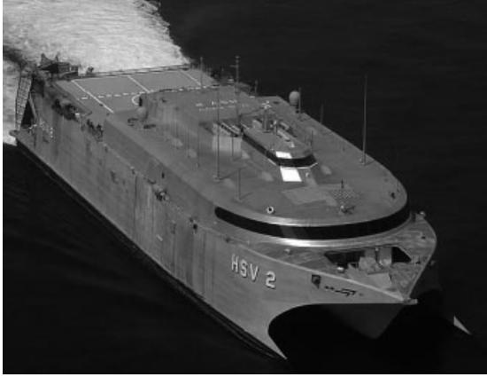
Figure 3. All aluminum high-speed vessel HSV-2, Swift.
