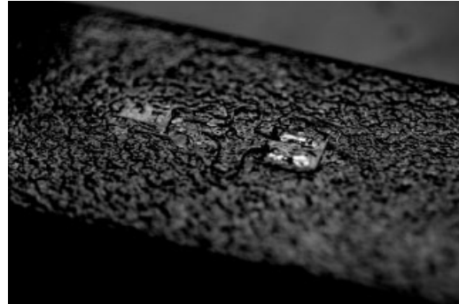
Figure 6. Photograph showing egress of lead wires from a piezoelectric transducer embedded in the ASP. Wires are shown connected to a solder tab.
