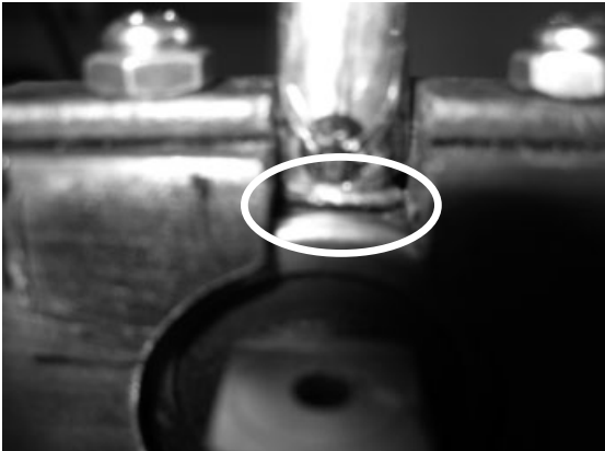
Figure 20. Initial circumferential crack in sway bar link under cyclic loading.
