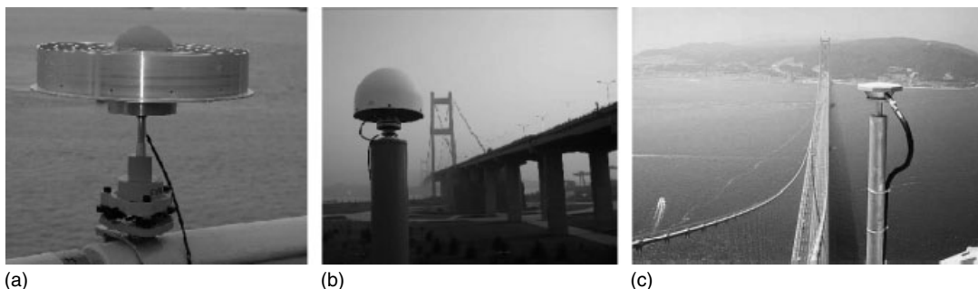
Figure 2. (a) A choker antenna; (b) a reference station set up on the Jingyin Bridge in China; (c) a monitoring station atop the Akaishi Kaikyo Bridge in Japan [photos courtesy of Leica Geosystems].
