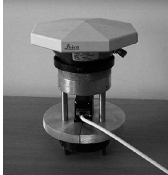
Figure 8. Device for integrated GPS antenna and a triaxial accelerometer.
