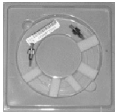
Figure 6. Typical fiber-optic sensors based on Bragg gratings (FBG).
