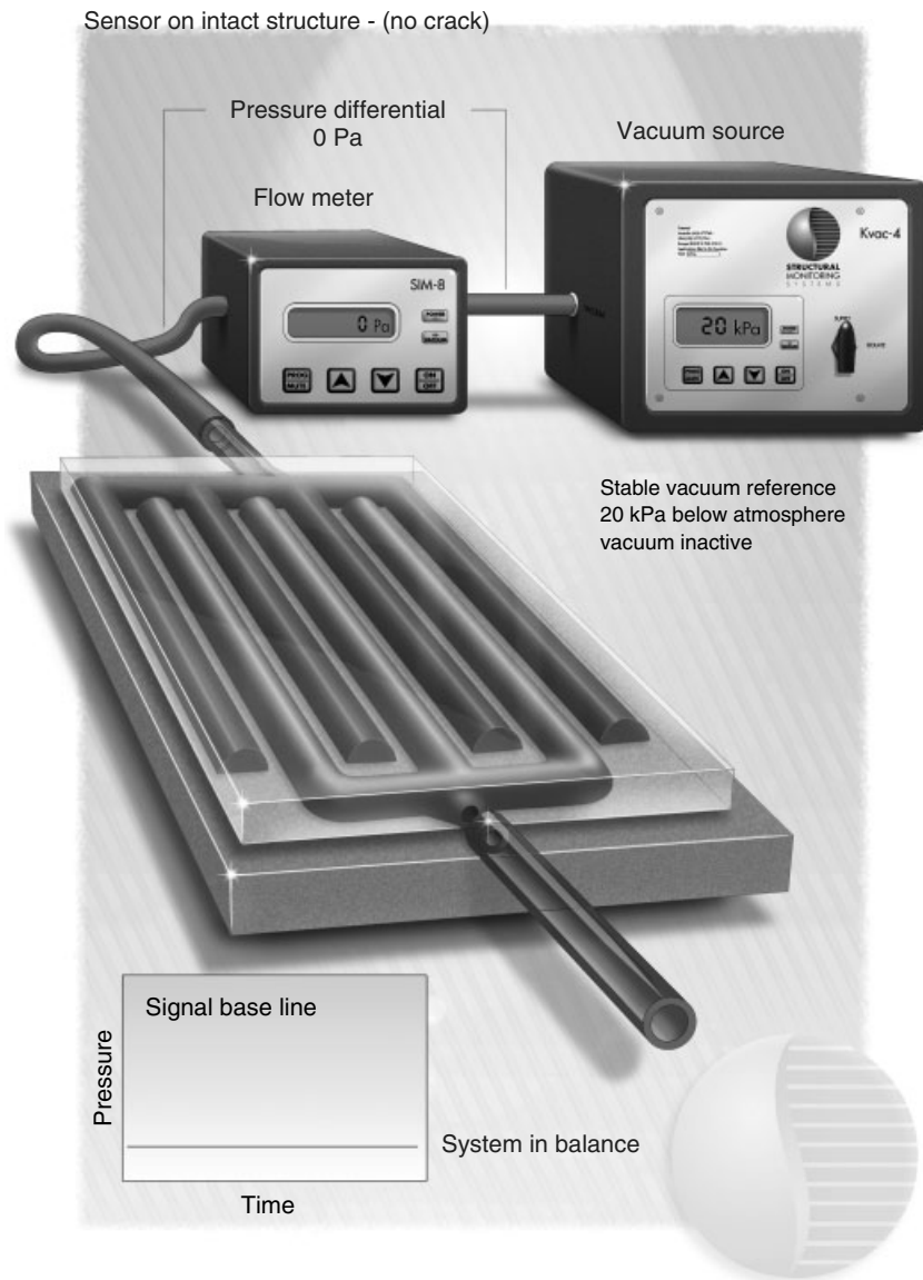
Figure 2. CVM™ system installed on an intact component.
