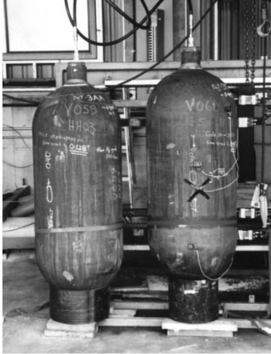
Figure 10. DOT spec 3AA tube undergoing cyclic fatigue. Ellipse shows position of crack near the center. MAE transducers are at the ends of small white wires. A 3T tube, seen at the right, was also tested. Good crack growth data were obtained.
