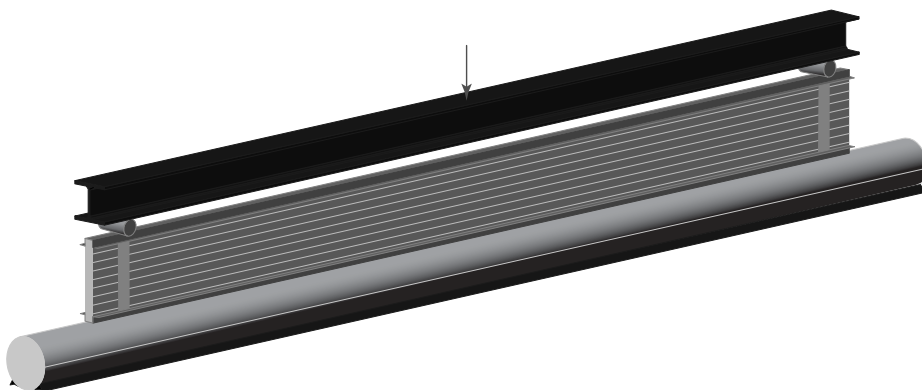
Figure 7. Constant continuous loading by means of the hydraulic principle.
