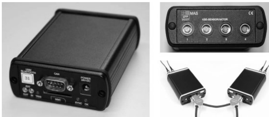
Figure 13. Four-channel sensor/actuator nodes for SHM of piping systems. The nodes can be combined to a multichannel measuring system that can be used for both active and passive monitoring. The present nodes are based on a CAN–Bus interface but wireless interfaces are also under development. Details of the hardware implementation can be found in Section 4 and in [13]. [Reproduced with permission from Ref. 13. © SPIE, 2007.]
