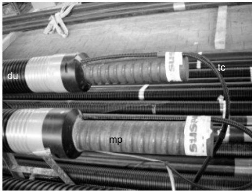
Figure 5. Critical points are splice joints (left) and cable egress points (right) in heavy steel anchors (mp, micropile/anchor steel; du, duct; tc, transmission cable). Photo: BAM.
