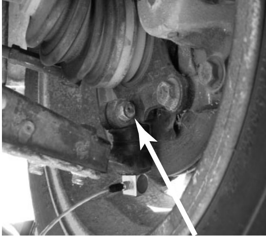
Figure 17. Ball joint connecting lower control arm to the steering knuckle.
