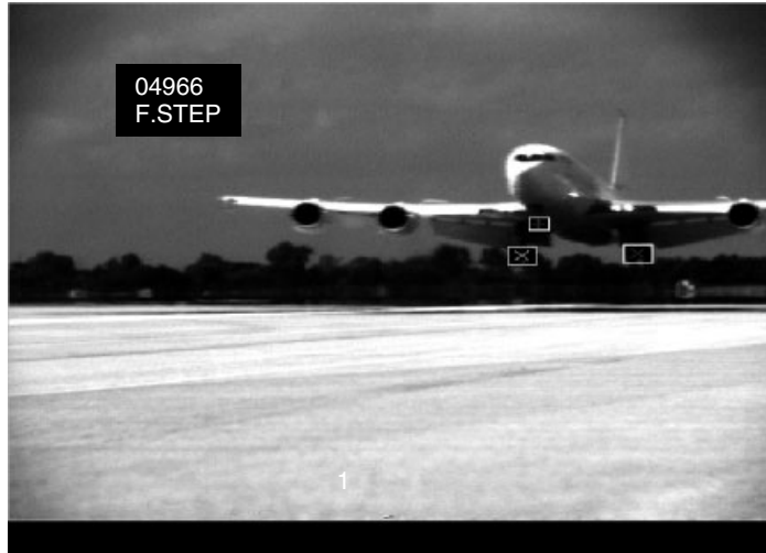
Figure 7. Video image of transport aircraft showing tracking windows used to extract analysis data.
