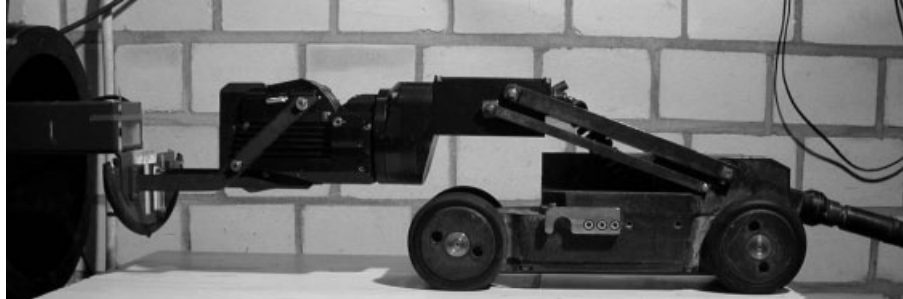
Figure 2. Camera lafette with elevated weir (on the left side).
