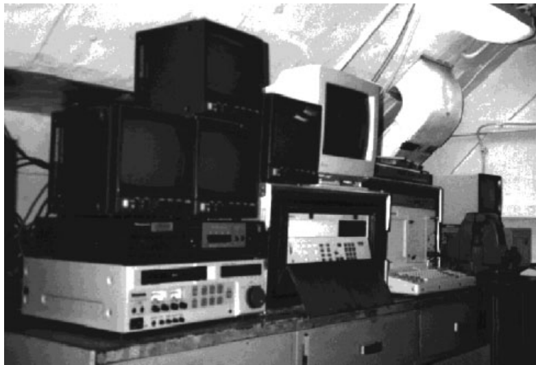
Figure 2. NAALDAS video system, data-acquisition hardware aboard aircraft carrier.
