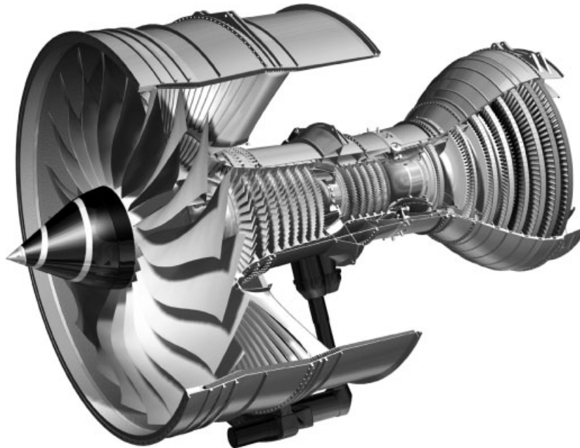
Figure 1. Aircraft gas turbine engine cross section.
