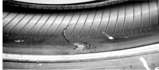
Figure 3. MEMS accelerometer bonded to the inner liner of the tire using silicone rubber (image from Apollo final report [3]).
