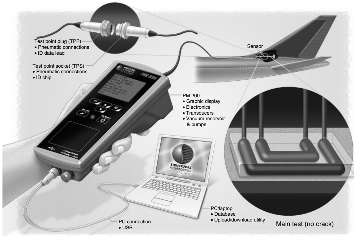
Figure 7. CVM™ check of the periodic system on an intact surface.
