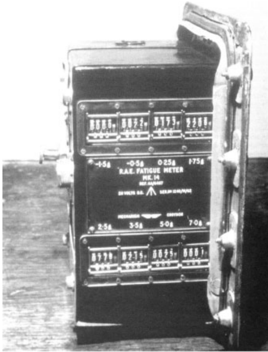
Figure 3. Acceleration exceedance monitoring system introduced in the Royal Air Force in the 1950s.
