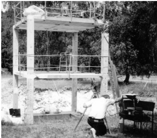
Figure 9. Experimental reinforced concrete structure under seismic-type loading.
