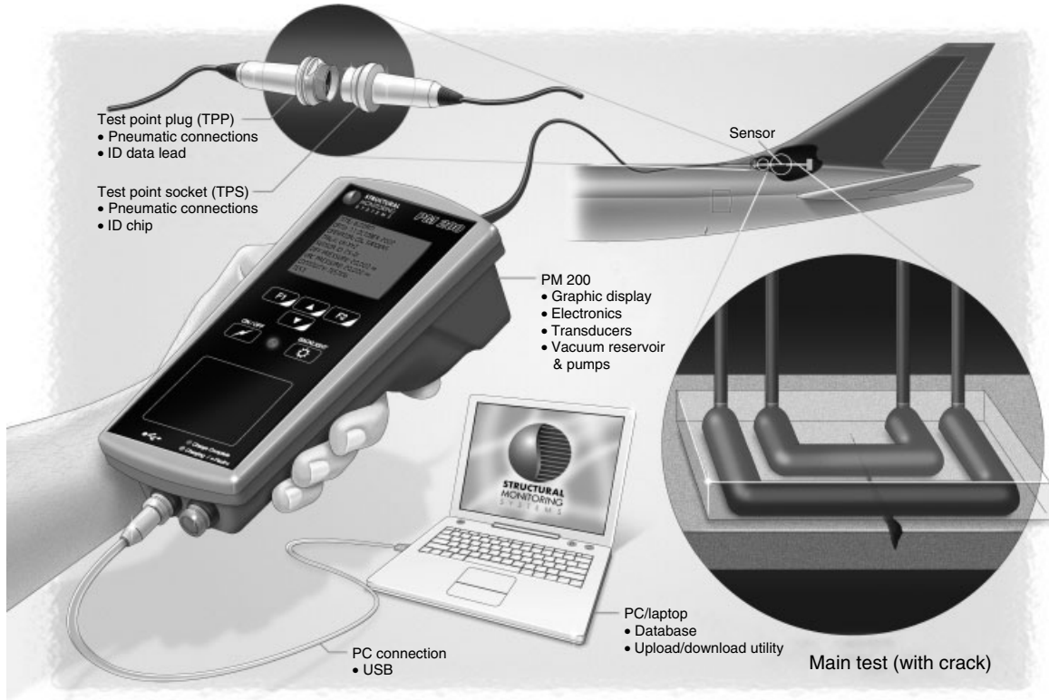
Figure 8. CVM™ check of the periodic system on a cracked surface.
