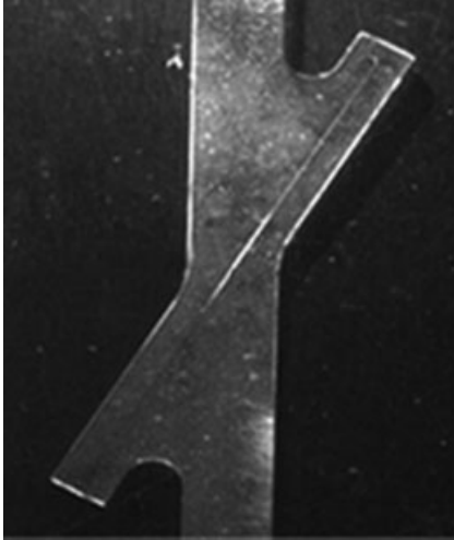
Figure 8. Geometry of cruciform specimen for fiber–matrix interface strength test. The white line at the center of the specimen reveals interface failure away from free-edge stress field.
