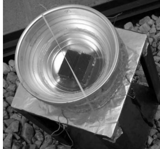
Figure 4. Experimental setup of the solar harvesting system.
