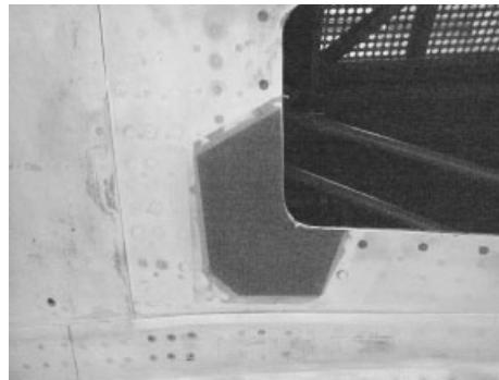
Figure 7. Composite repair patch applied to an aircraft fuselage.
