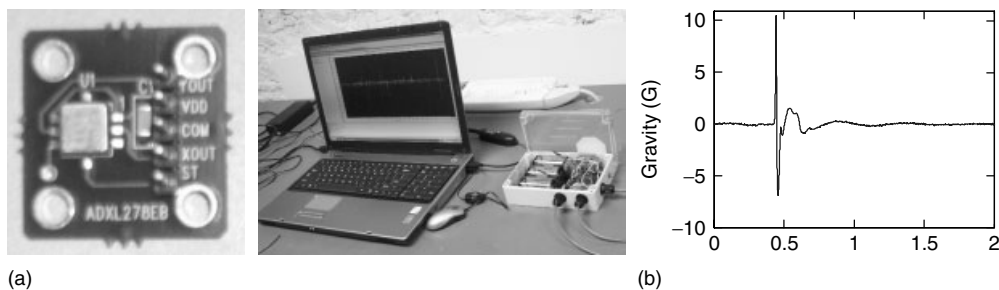
Figure 17. Wireless data-acquisition system with eight MEMS accelerometers: (a) MEMS accelerometer/board, battery-powered wireless module, laptop computer with bay station and (b) one channel response due to a shock input. This system was assembled at the University of Cincinnati using commercial components. Continuous accelerometers can be used to allow 32 or more individual MEMS accelerometers to be used with this system.
