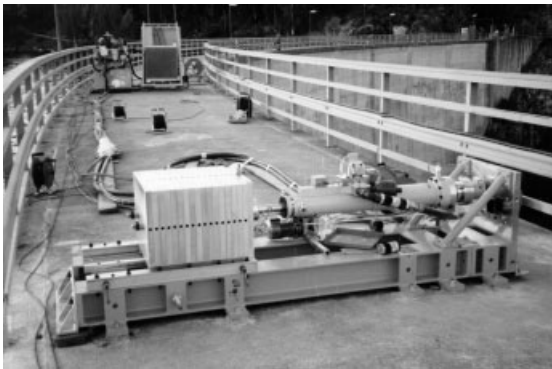
Figure 18. The servohydraulic shaker fixed to the Norsjö dam crest. In the background, the air-sprung hydraulic power pack to the left and the air cooler to the right.
