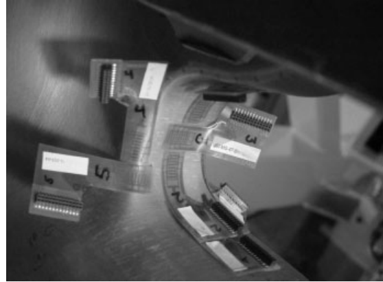
Figure 3. Jentek MWM-array sensors fixed to the landing gear structure. [Reproduced with permission. © Messier-Dowty Inc.]
