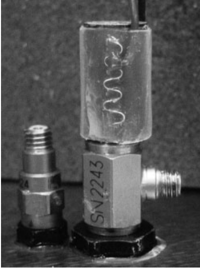
Figure 4. Piezoelectric sensor/actuator pair for SHM. [Reproduced with permission from Ref. 72 & 73, © SPIE, 2000.]
