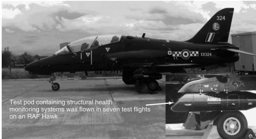
Figure 5. Recent flight tests of optical sensors aboard a Hawk military jet. A group of SHM systems, including fiber-optic strain gauges were contained in an underwing pod during flights.
