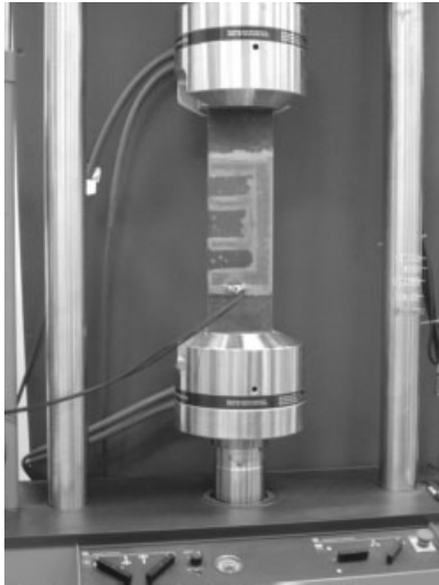
Figure 22. Steel plate with composite doubler, engineered flaws, and PZT sensor network undergoing fatigue tests.
