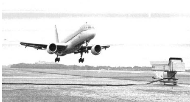
Figure 1. Video camera in operation during commercial landing parameter survey.
