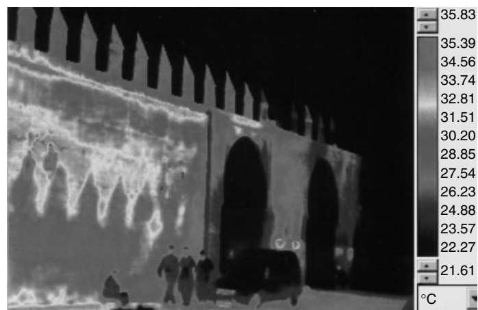
Figure 3. Thermal diffusivity characteristics of the front face of the royal palace in Fès Marocco.
