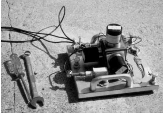
Figure 8. 3-D accelerometer response measurement point fixed to the dam crest.
