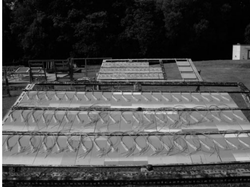
Figure 13. Test coupons experiencing hot/wet tropical conditions. [Courtesy of DSTO].
