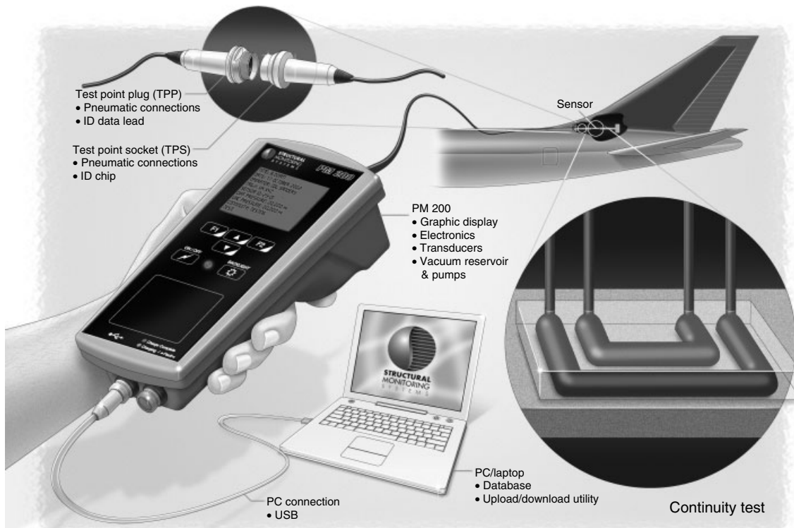
Figure 6. Continuity check of the periodic system—ensuring the sensors are not blocked.
