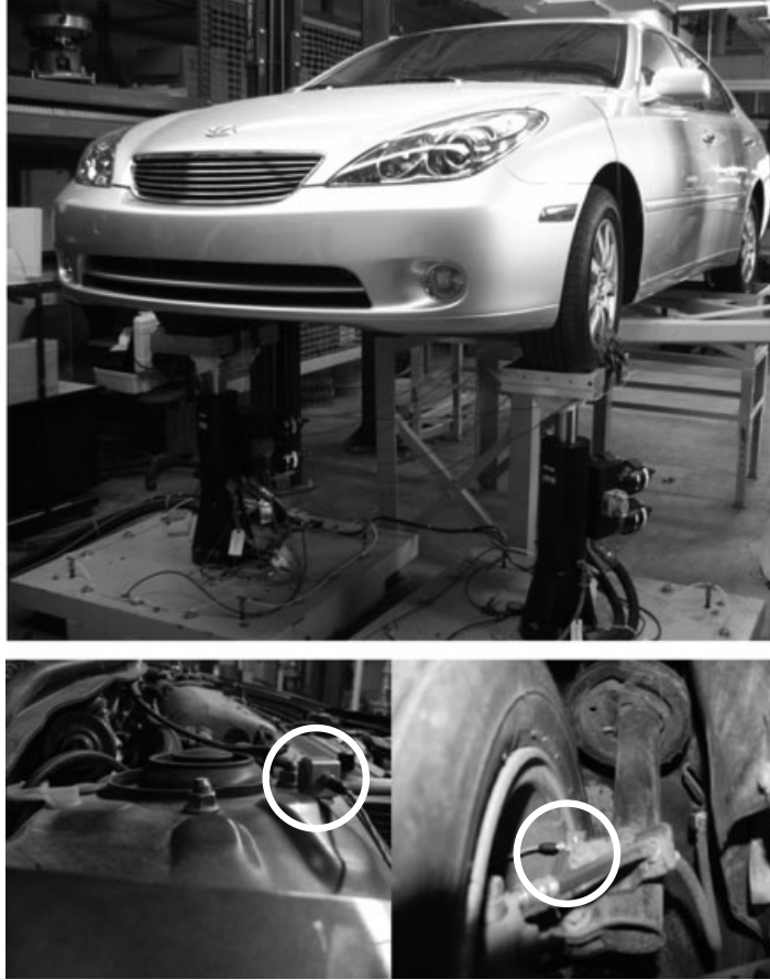
Figure 6. Two-post shaker setup and accelerometer locations.
