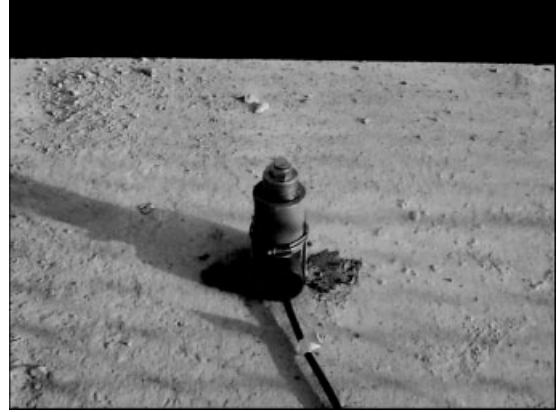
Figure 11. Hydrodynamic pressure sensors arranged on deck.
