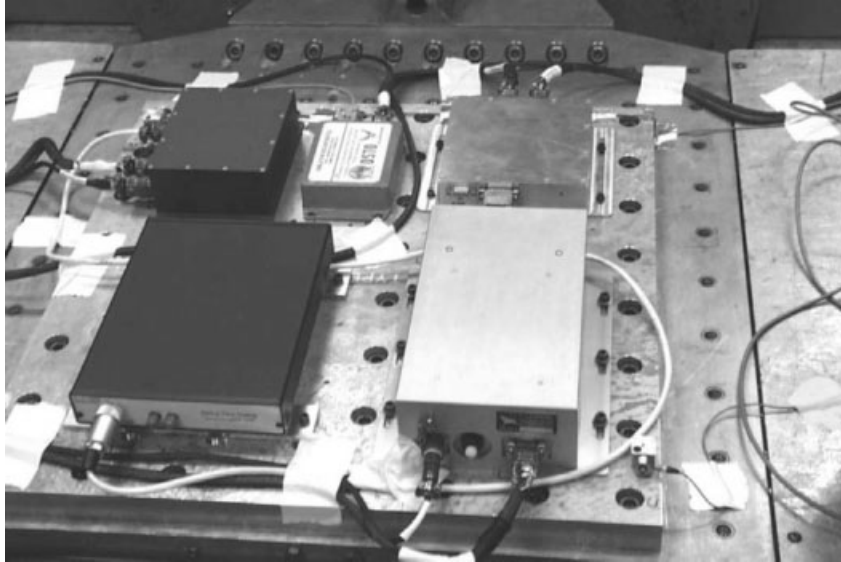
Figure 1. Boeing’s ASIMS data-acquisition system and battery integrated with the Luna fiber-optic sensor signal conditioning system.
