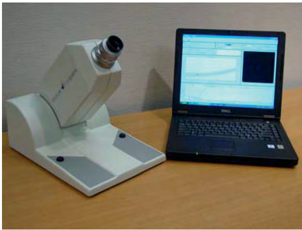
Figure 4 The C-Quant instrument from Oculus for measuring the amount of straylight in patient eyes.
