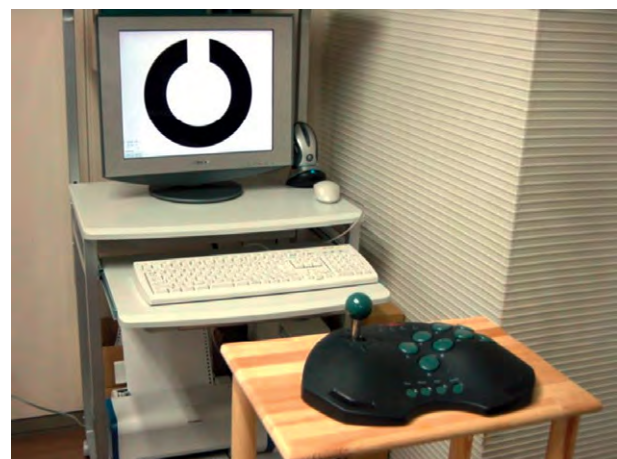
Figure 3 Functional visual acuity (FVA) system. This is a compact device developed to measure changes in continuous visual acuity over time.
