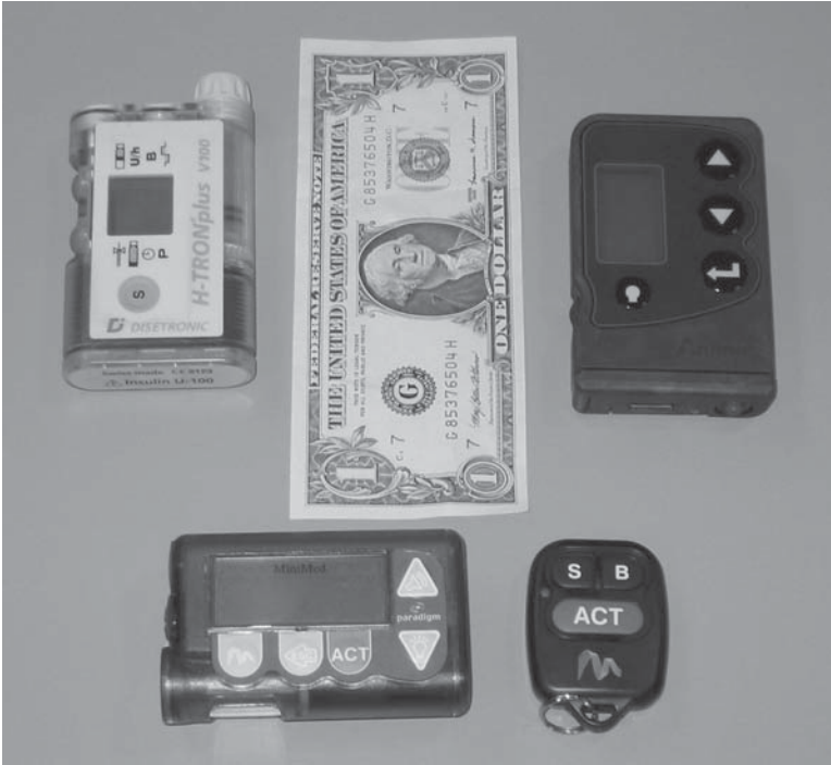
Fig. 1. Insulin pumps compared in size with a dollar bill. From left to right: Disetronic, Medtronic MiniMed, and Animas pumps.
