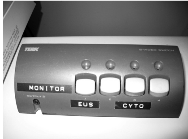
Figure 3.5 The endosonographer can maintain control over the image displayed on the room's primary monitor using a switcher box. In this case, the box receives input from both the EUS processor and a video microscope.
