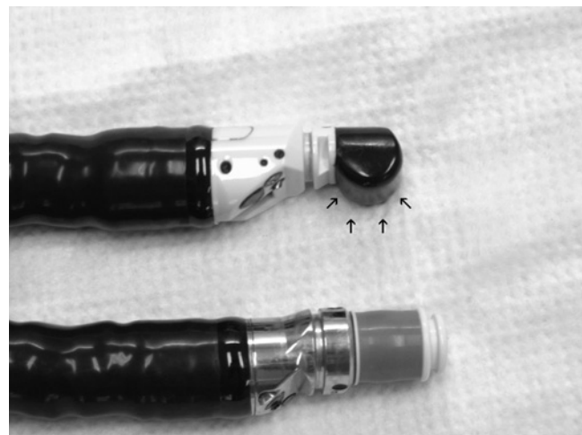
Figure 3.1 A linear array echoendoscope ( top ) and an electronic radial array (also called transverse array) echoendoscope ( bottom ). The piezoelectric crystals on the linear array echoendoscope are arranged along a single curved surface ( arrows ). On the electronic radial array echoendoscope the crystals are arranged as a band around the side of the instrument's tip.
