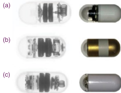
Figure 1.13 Examples of the internal and external structure and components of the main capsule systems. Both (a) and (c) use radiofrequency (RF) transmission and dedicated RF receiver arrays for wireless video recording, whereas (b) uses the body to transmit the video to the recorder. Standard electrodes in an array are used to pick up the video signals.
