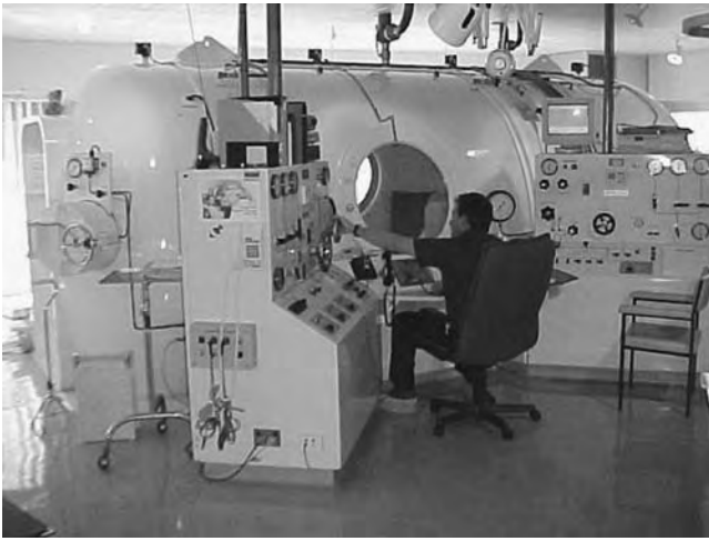
Figure 53.1. Multiplace hyperbaric chamber. The multiplace chamber is compressed with air and the patient breathes 100% oxygen via mask or hood inside the chamber. (Photo courtesy of Dick Clarke.)
