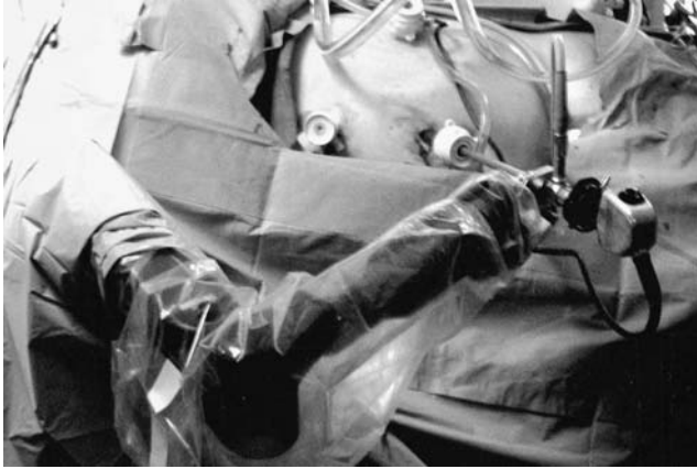
Fig. 1. AESOP (automated endoscopic system for optimal positioning) camera holder enables a single surgeon to perform a laparoscopic procedure
