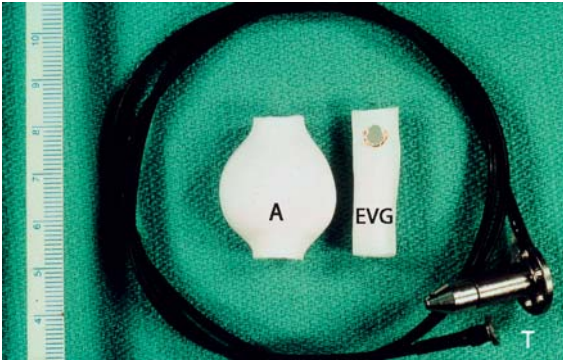
Fig. 2. Artificial aneurysm made of PTFE with an EVG containing a punched hole with a radio-paque marker. The EVG is placed inside the aneurysm and sutured to it at both ends. A pressure transducer tip is sutured to the aneurysm wall. The transducer has a cable and a connector that is placed in a subcutaneous tunnel and guided out at the neck of the animal. A: aneurysm; T: pressure transducer tip; EVG: endovascular graft
