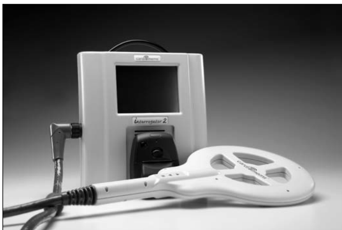
Figure 29-2. CardioMEMS interrogator 2™ monitor system and display with handheld antenna attached by cable. When used in the operating room, the racquet-shaped antenna is sheathed in a sterile plastic sleeve.
