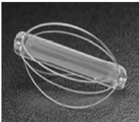
Figure 27-4. Image of an implantable EndoSure™ wireless aneurysm pressure sensor measuring 30 × 5 × 1.5 mm (CardioMEMS, Atlanta, GA). (Reprinted from Okhi T, Ouriel K, Silveira PG, Katzen B, White R, Criado F, and Diethrich E. Initial results of wireless pressure sensing for endovascular aneurysm repair: The APEX Trial – acute pressure measurement to confirm aneurysm sac EXclusion. Journal of Vascular Surgery . 45: pp. 236–242. Copyright 2007, with permission from The Society for Vascular Surgery.)
