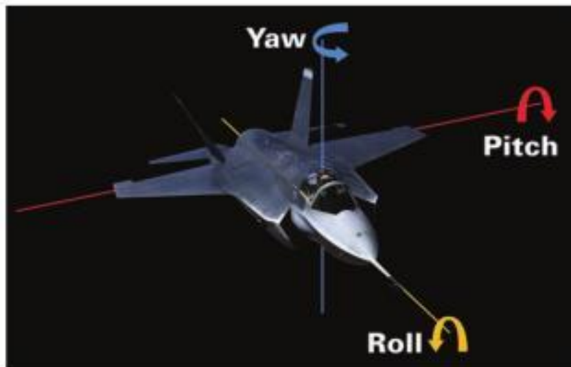
Figure 4.12 Three-dimensional movement in space is defined by translation (forward/backward, up/down, right/left) combined with rotation about three perpendicular axes (pitch, yaw, and roll). A complete description of a plane's orientation in space requires consideration of all six attributes. (Reprinted from Ackerman, J.L., Proffit, W.R., Sarver, D.M., Ackerman, M.B., Kean, M.R. Pitch, roll, and yaw: Describing the spatial orientation of dentofacial traits. Am J Orthod Dentofacial Orthop Vol. 131, 2007, with permission from the American Association of Orthodontists.)
