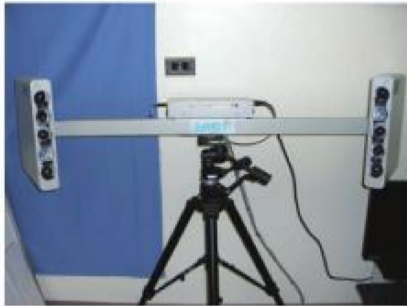
Figure 4.3 The 3dMD stereo photogrammetric scanner (3dMD, Atlanta, Georgia). It consists of an array of digital cameras used to perform surface imaging of the patient's face. A quick scan will generate a clinically accurate three-dimensional digital model of the patient's face.
