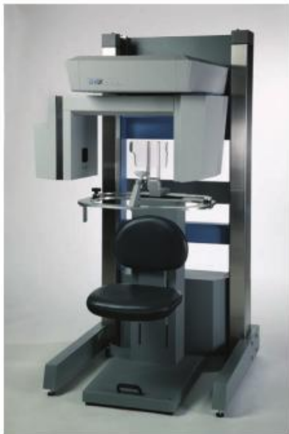
Figure 4.6 The i-CAT cone-beam computed tomography (CBCT) system. The CBCT technique involves the patient seated in the scanner with the x-ray source and reciprocating detector synchronously moving around the patient's head in a single 360-degree scan. (Image courtesy of Imaging Sciences International, Inc., Hatfield, Pennsylvania, and their public relations firm, Gregory FCA Communications, Ardmore, Pennsylvania).
