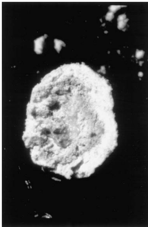
Fig. 13.1. Cross section of a water dispersible granule showing enclosed infective juveniles of Steinernema carpocapsae .
