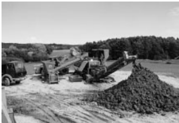
Fig. 10.2 Soil preparation unit type 'mole'.
