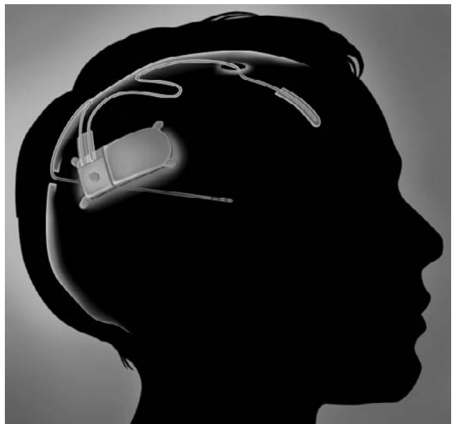
FIGURE 17-3. Schematic of the NeuroPace RNS™ neurostimulator, depth and strip leads.
