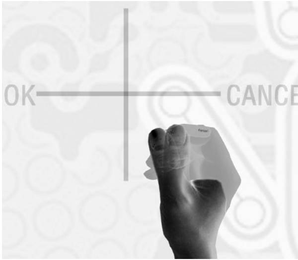
Fig. 8. This design takes the first joint of forefinger as the touchpad of a laptop computer. Clicking on the left side is OK, and clicking on the right side is cancel.
