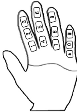
Fig. 7. This number keyboard can be worn on a hand, and takes person's finger joint as keyboard's key position, switching twelve basic key positions, and the functional key position, can realize all the function of input
