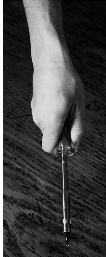
Figure 11-7 A power grasp. The object is held firmly in the palm of the hand. The wrist is ulnarly deviated to align the hand with the longitudinal axis of the tool.
