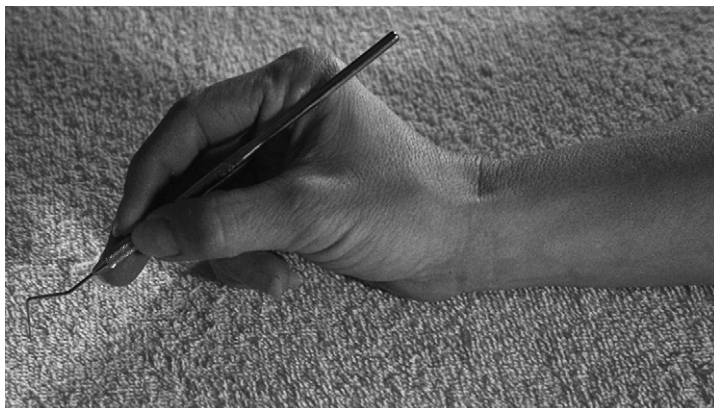
Figure 11-15 Handle size for precision tools. A modified palmar (or tripod) grasp is commonly used for precision work. Precision tools have a small diameter and smooth tip for accurate work.
