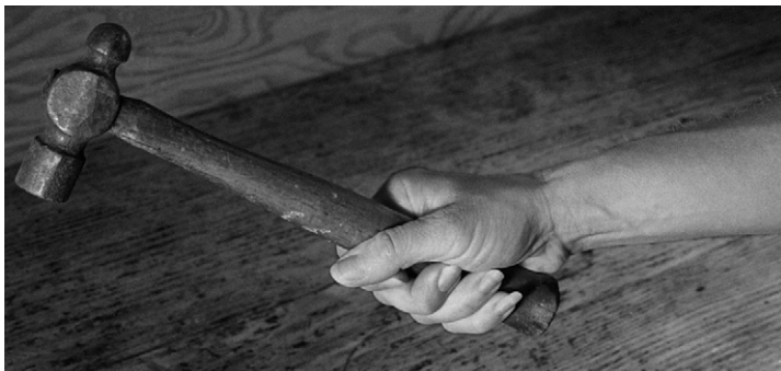
Figure 11-13 Handle size for a cylindrical tool. Both distal interphalangeal (DIP) and proximal interphalangeal (PIP) joints should be in midflexion.
