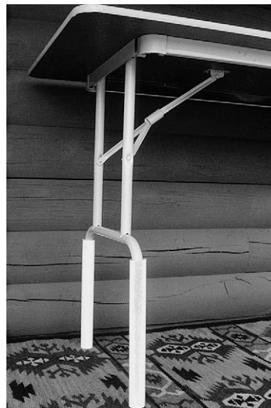
Figure 20-6 Lengths of 1 \frac{1}{4} -inch PVC pipe used to raise a conference table to proper height for cutting.
