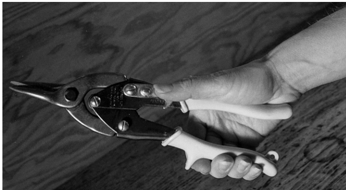
Figure 11-14 Handle size for a two-handed tool. Proximal interphalangeal (PIP) joints should be in midflexion at the application of force.
