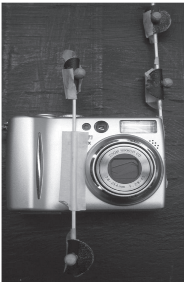
Figure 1. Photo of the camera used and the markers attached to the camera.
