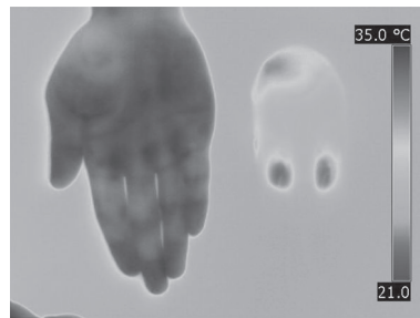
Figure 5. The IR camera image of hand and computer mouse after static holding the mouse for three minutes. The contact areas of hand and mouse interface were mainly at index and third finger area and posterior palm area.
