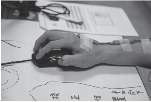
Figure 9. The static holding position taking with a regular camera. In this photograph we can only see the outside feature of gripping a mouse but not the real contact area.
