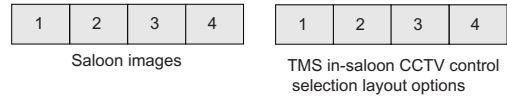
Figure 6. The linear layout of camera images on CCTV display (left) and matches with the selection panel on TMS (right). The numbers represent sections of the car instead of camera numbers. The camera numbers are transparent to the operators and a translation matrix was developed for the engineers based upon what the operators wanted to see on the interface.
