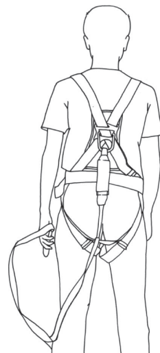
Figure 1. Incorrect position of back D-ring.
