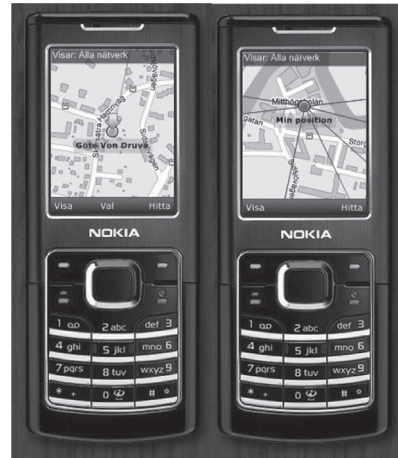
Figure 1. Left: User's own position is illustrated by a blue sphere and the lines drawn between the user and the people who are in the user's surrounding area Right: When a person is selected, this is illustrated with an orange arrow pointing at the person.
