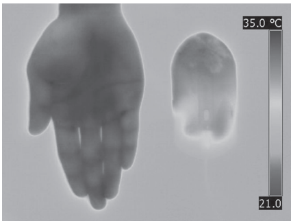
Figure 6. The IR camera image of hand and computer mouse after dynamic web browsing for 15 minutes. The contact areas of hand and mouse interface were mainly at index and third finger area and posterior palm area.
