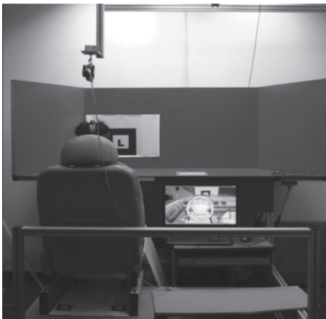
Figure 8. Hardware system for vehicle interior ergonomic evaluation.
