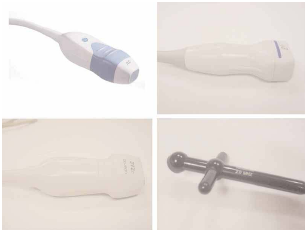
Fig. 1. Adult transthoracic echocardiography transducers generally range between 2 and 7 mmHz, with lower frequency transducers—2.5 and 3 mmHz—being the most commonly used. Higher frequency transducers are routinely used in pediatric echocardiography and transesophageal echocardiography. They provide increased resolution, but decreased penetration. The dedicated Doppler transducer (bottom right) is a nonimaging probe. These are standard components on modern echocardiography machines.
