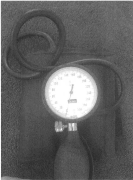
Figure 2.7 • The traditional sphygmomanometer. Portable versions, such as this, use dials. Desktop systems tend to still employ a mercury column to indicate pressure.
