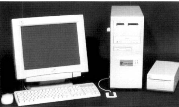
Fig. 17.7 The Trophy Radiovisiography® (RVG) real-time digital imaging system where the CCD sensor is connected directly to the computer.
