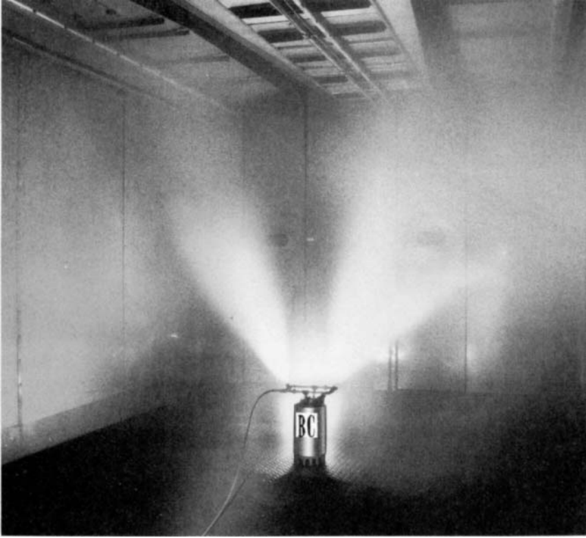
FIGURE 12.4. A portable atomizer that covers all stainless-steel surfaces in a smoke-house and reduces cleaning time by 60 to 75%. (Courtesy of Birko Chemical Corporation.)
