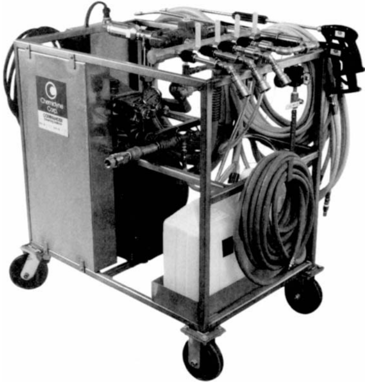
FIGURE 7.1. A portable high-pressure, low-volume cleaning unit that can be used without a centralized system. This unit has racks for hoses, foaming compounds, and cleaning compounds, and has two rinse stations and a sanitizer unit. Two workers can use the unit at the same time to prerinse, clean, postrinse, and sanitize. This equipment can also apply foam if the spray wand is replaced with a foam wand accessory. (Courtesy of Chemidyne Corp.)
