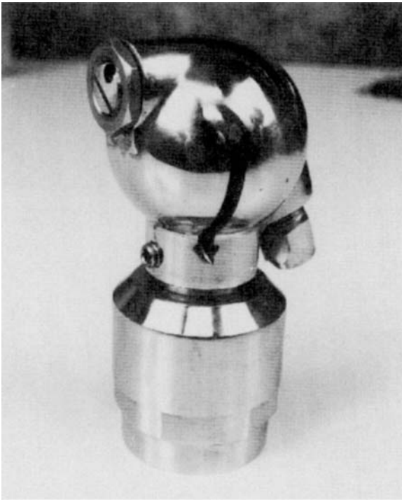
FIGURE 7.8. A spray ball that mechanically cleans large and small tanks. It consists of a stainless-steel head on a self-cleaning alkali- and acid-resistant ball race. The spherical head has a wide-angle nozzle and is slotted to saturate surfaces in every direction. An offset jet spins the ball vertically at adjustable speed. (Courtesy of Oakite Products, Inc.)
