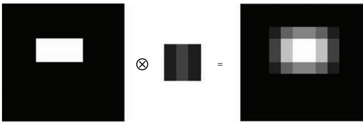
FIGURE 5.26 An example of the convolution operation between two 2-D grids of numbers (top), or alternatively, the same example is shown as images (bottom). The center portion of the figure shows the mathematical operation of the 2D convolution, and the result shows how: in this example, the result is a spatial smoothing or blurring of the original image.
