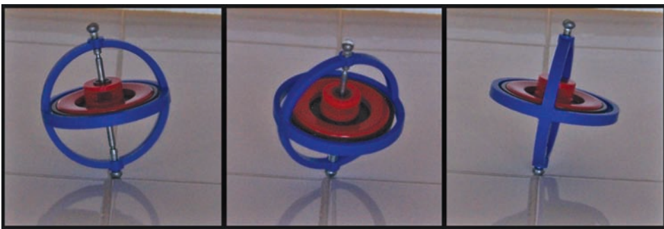
FIGURE 3.5 A gyroscope with its heavy red disc at the center spinning rapidly on its axis. The sequence of pictures shows the gyroscope wobbling, or precessing , due to its angular momentum, instead of simply falling over under the force of gravity.
