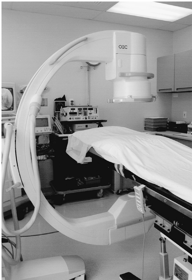
FIGURE 68-8 A conventional undercouch fluoroscopy arrangement wherein the x-ray tube is located beneath the fluoroscopy table and the image intensifier is above the table.
